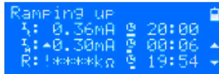
*Fig 19. Resistance too high during ramp-up*
