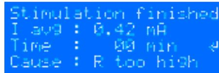
*Fig 20. Stimulation terminated because of high resistance*
